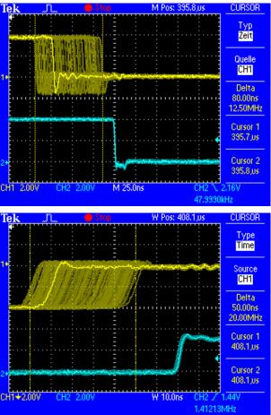
The cleaned and jitter-freed signal can be used as reference clock for any application, without any problem. The signal processed by SteadyClock is of course not only used internally, but also available at the Micstasy's word clock output. It is also used to clock the digital outputs MADI and AES/EBU.
