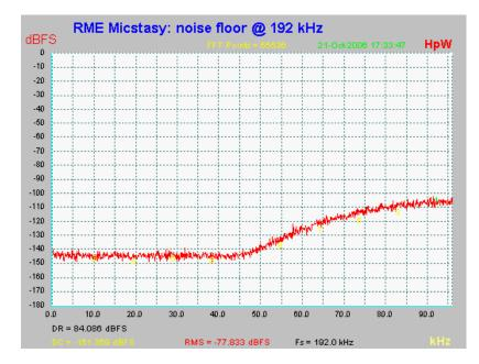
As can be seen in the above picture, the noise floor stays fully unchanged up to 45 kHz. With sample rates up to 96 kHz the noise shaping completely happens outside of the transmission range.
